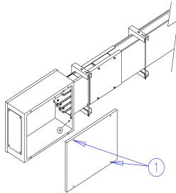
b) Unscrew the screws (1) and remove the lid.
