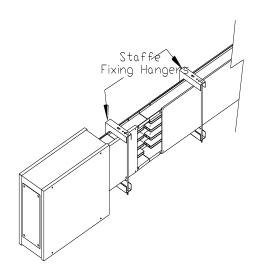
a) Fix the support and mount the feed unit to the first bus way element as explained into "Assembly instruction line and GDA joint"; we suggest to support the feed unit body with another support.
