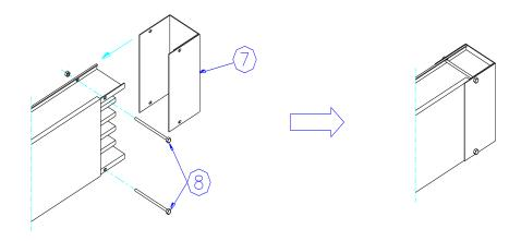
g) Fix the end cap (7) pushing until the corresponding holes match and tight the four screws (8).
